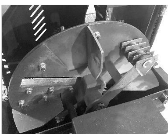
Disc wheel with blades and knife
