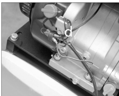
Connecting the safety circuit (EMERGENCY STOP)
