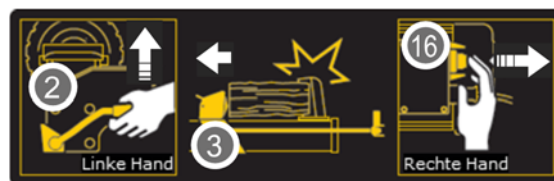
Fig. Two-hand control: Pressure plate retracts
